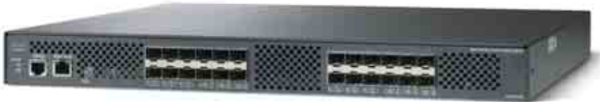
High density design with 24 ports in 1RU height can help save rack space
